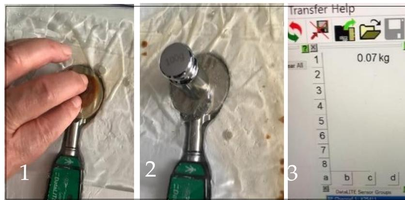
**Figure 3.** Effect on pressure transmission via restored layer of fluid. (1) Manipulations for breaking and dissolving the caramel plug; (2) the caramel plug is dissolved and the 0.1 kg weight is positioned over the bag; (3) load of 0.07 kg registered by the system on computer screen.
