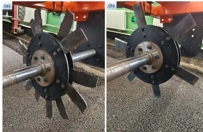
**Figure 8.** Stubble-cutting blade: (a) BSCD; (b) TPSB.
