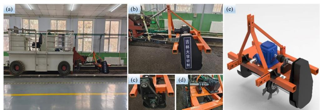
**Figure 6.** Soil bin test equipment: (a) Soil bin tester system; (b) Power transmission system; (c) Sprocket transmission; (d) Gearbox; (e) Three-dimensional design drawing of the power transmission system.
