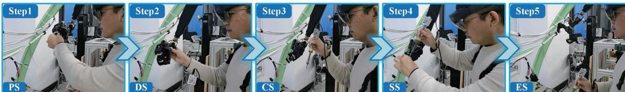
Figure 12. Experimental operating procedure for soldering tasks. Step 1: The SRL grabs the electrical connector and enters dragged motion mode. Step 2: The operator drags the end of the SRL to a suitable position. Step 3: The SRL end follows the soldering iron to adjust the angle. Step 4: The operator completes the soldering task. Step 5: The soldering task is completed, and the SRL returns to the preset position.
