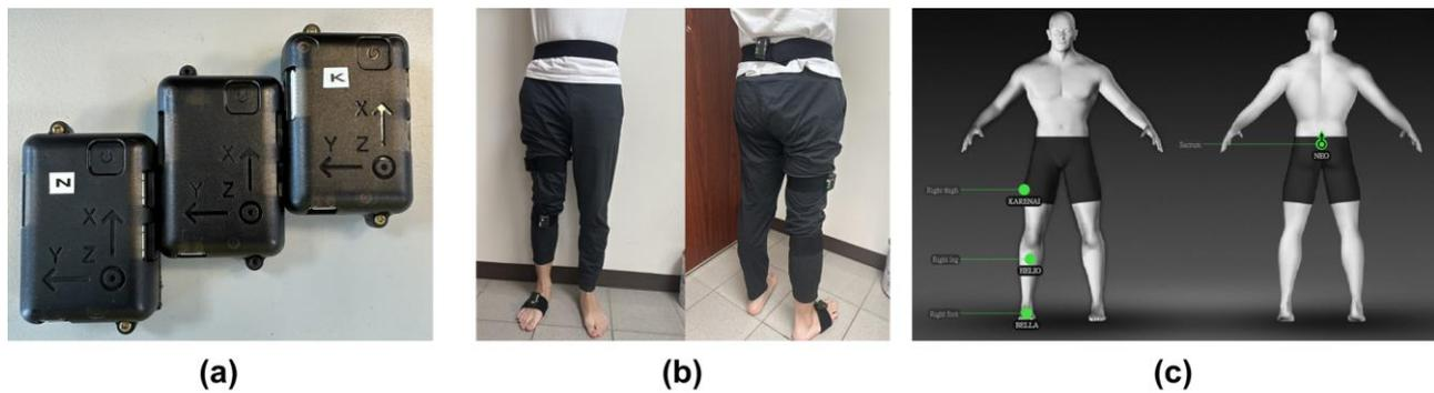
**Figure 1.** (a) The IMU equipment: NGIMU; (b) the front and back view of the subject wearing IMU sensors; (c) the setting of IMU sensors displayed in the iSen 3.0 analysis system.
