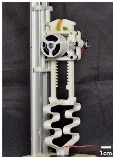
**Figure 1.** The proposed hopping robot. The robot has a height of 143 mm and weight of 46 g.
