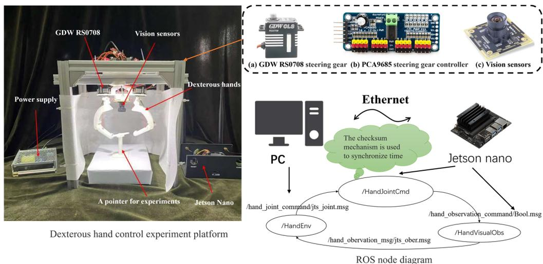
**Figure 11.** Scheme of the experimental platform.
