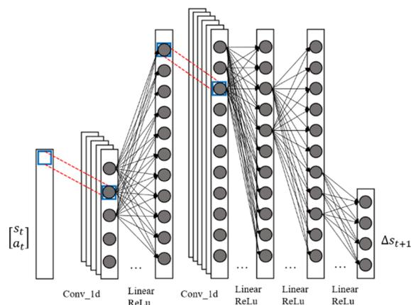
Figure 3. Generative network diagram for the dexterous hand.
