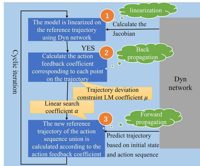
Figure 7. Steps for adaptive trajectory planning.
