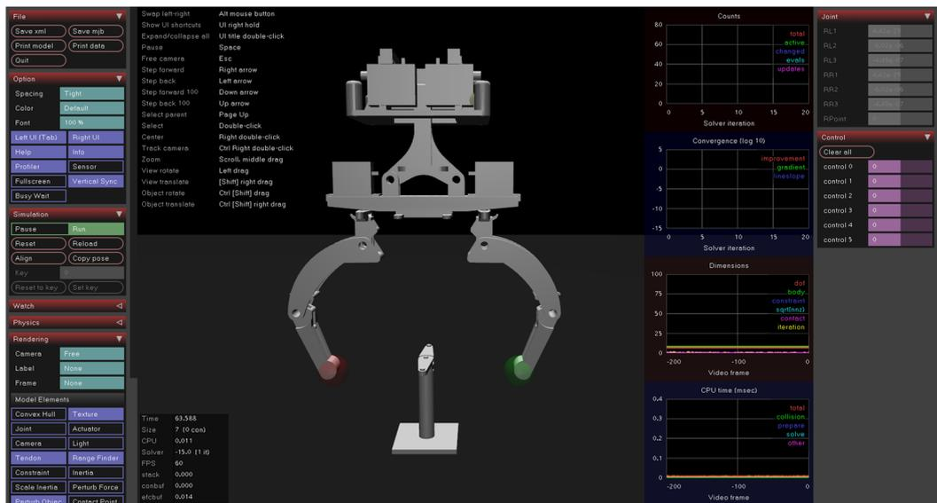
Figure 8. Simulation environment of a two-fingered hand.
