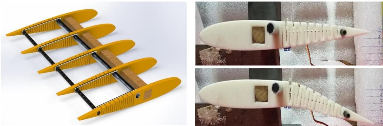
Figure 3. Detailed design of internal morphing structure and mechanism.
