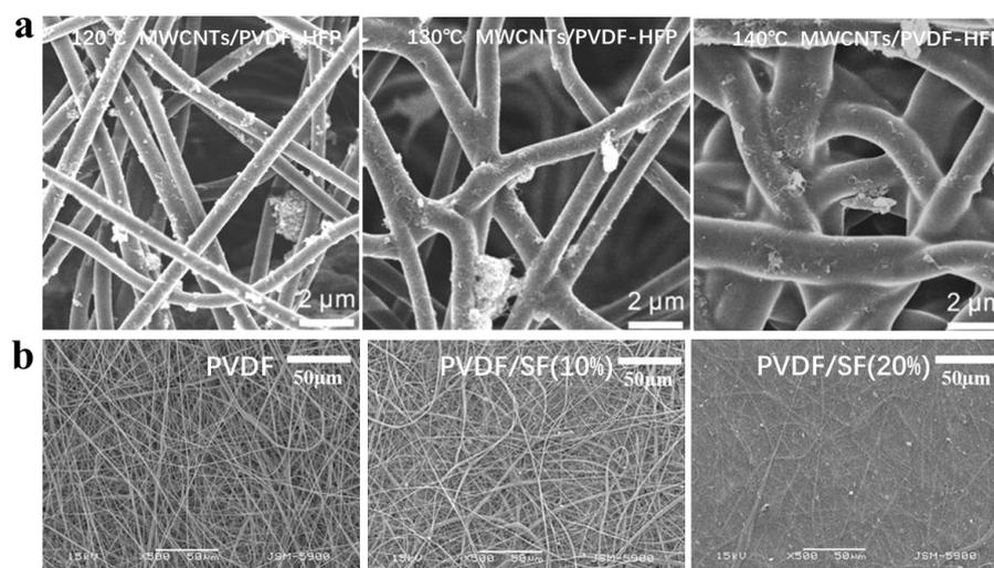
**Figure 3.** (a) SEM images of PVDF-HFP nanofibers with MWCNTs added after annealing treatment under 120, 130, and 140 °C for ten minutes, respectively [86]. Copyright 2019 American Chemical Society. (b) SEM images of PVDF/SF fibers added with 0%, 10%, and 20% filament protein nanofibers [87]. Copyright 2021 John Wiley & sons.
