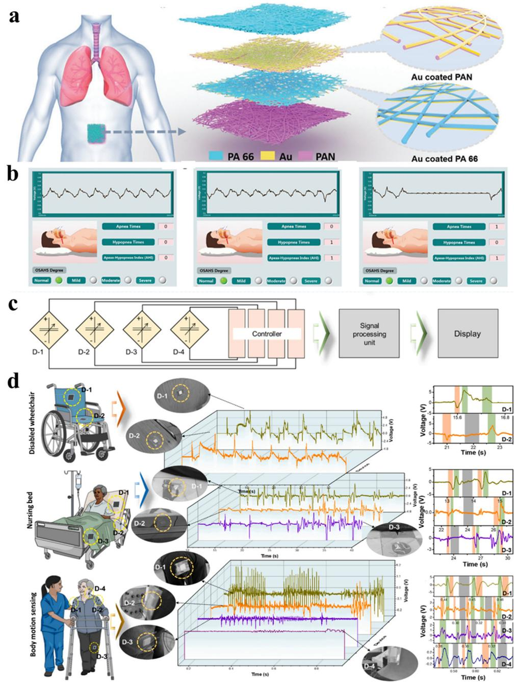
**Figure 8.** (a) An illustration of the structure of TENG-based SANES. (b) The sleep respiratory state judgment based on the OSAH diagnosis system [174]. Copyright 2021 Wiley-VCH. (c) Circuit diagram of health monitoring system connecting various TEHS devices to the monitor. (d) Integration of multiple TEHS in a wheelchair, nursing bed, and body for building health monitoring systems [175]. Copyright 2022 Elsevier.
