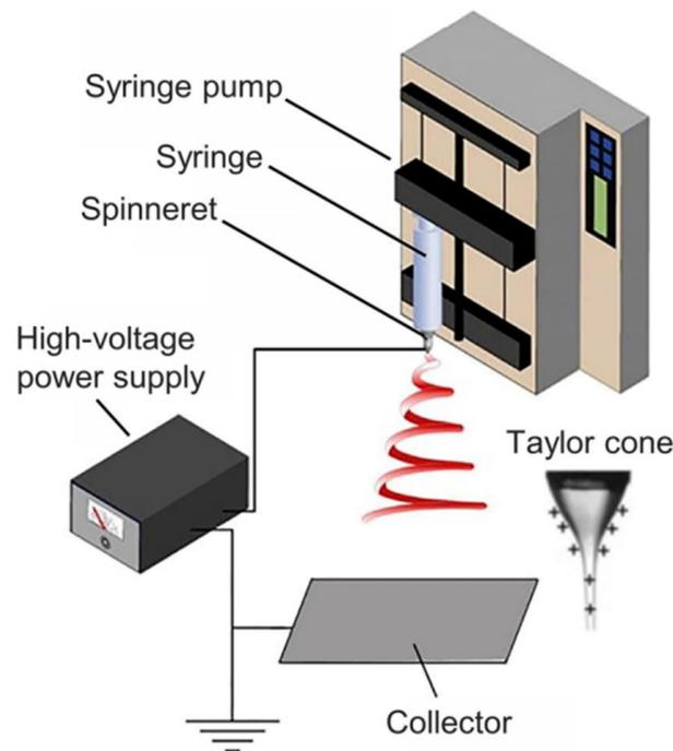
**Figure 2.** Illustration of electrospinning apparatus [23]. Copyright 2017 American Chemical Society.
