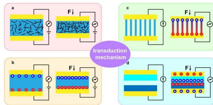
**Figure 6.** The illustration of four typical sensing mechanisms: (a) piezoresistive, (b) capacitive, (c) piezoelectric, (d) triboelectric sensing [104]. Copyright 2021 MDPI.
