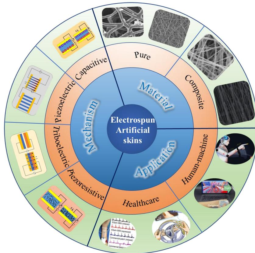
**Figure 1.** Summary of electrospun-based bionic artificial skin, which includes the material selection, working mechanism, and related applications.
