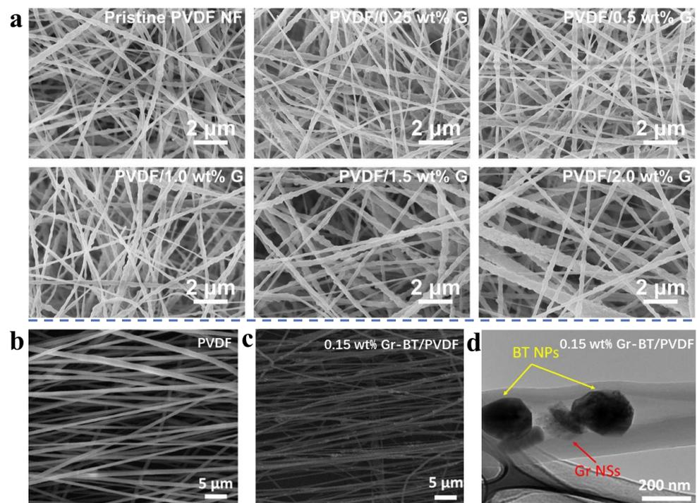
**Figure 5.** (a) SEM images for different GNS density (0–2.0 wt%) of electrospun PVDF/G composite nanofibers [98]. Copyright 2020 Elsevier. (b) SEM image of pure PVDF fibers. (c) SEM image of Graphene-BT/PVDF nanocomposite fibers with graphene concentration of 0.15 wt%. (d) TEM image of Graphene-BT/PVDF nanocomposite fibers with graphene concentration of 0.15 wt% [99]. Copyright 2018 Elsevier.
