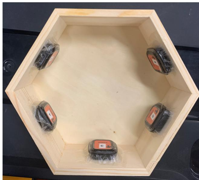
**Figure 2.** Apparatus for testing of drift under dynamic conditions.
