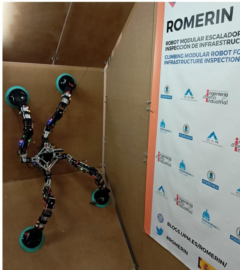
**Figure 1.** The ROMERIN robotic organism on vertical surfaces.
