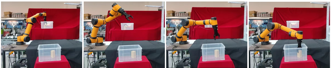
Figure 11. The path sequence of AUBO–i5 when executing the picking task.
