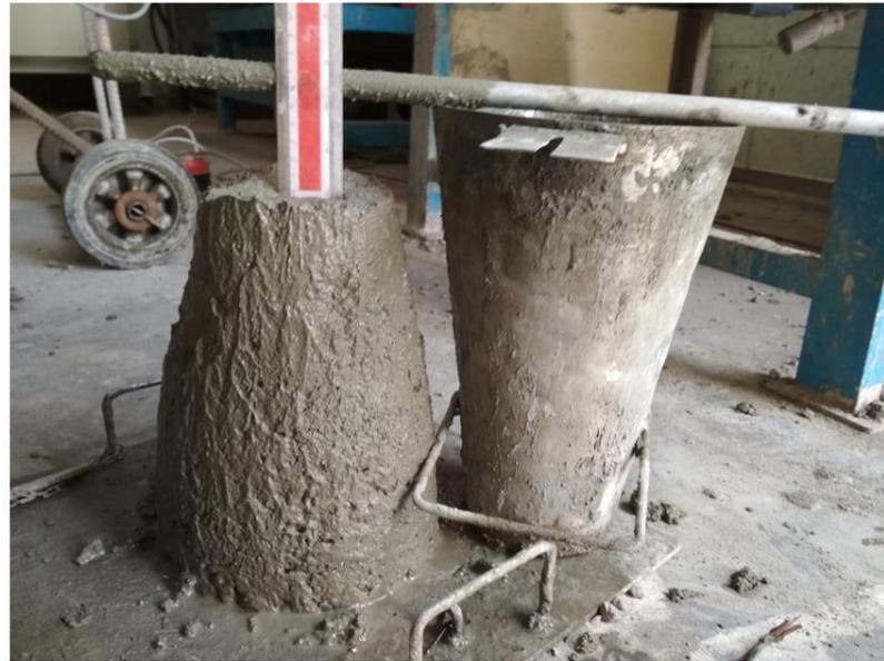
**Figure 4.** Fresh concrete' slump test.
