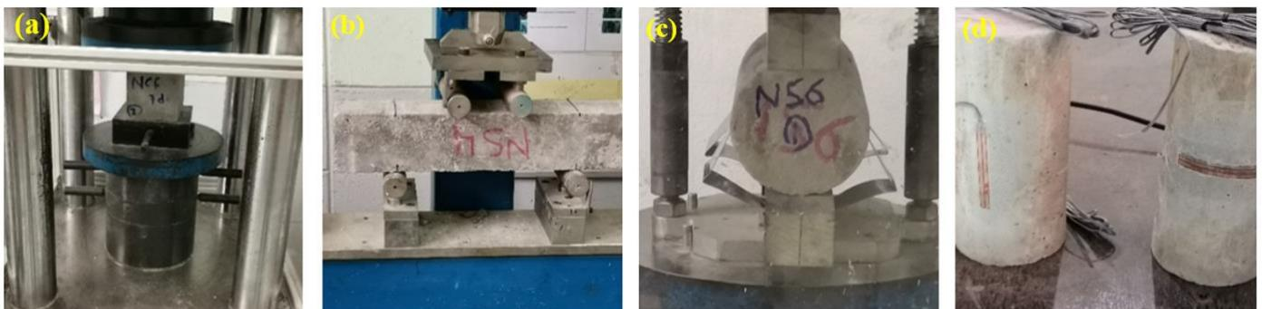
**Figure 5.** Mechanical tests of specimens' (a) compressive strength, (b) flexural strength, (c) splitting tensile, and (d) modulus of elasticity.
