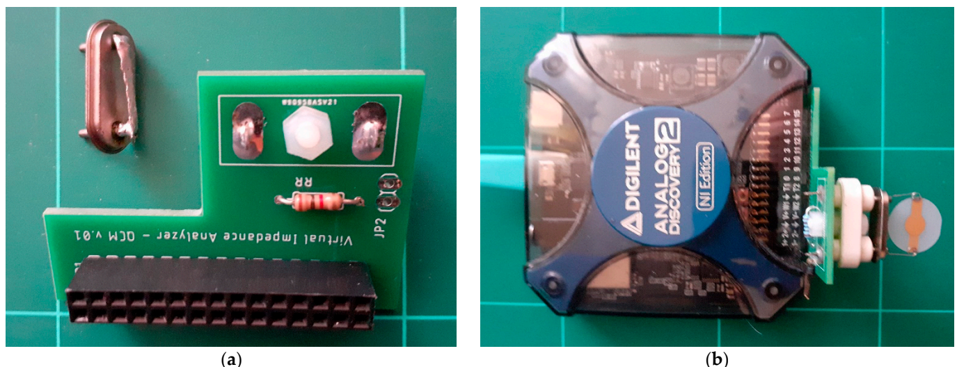
Figure 2. The virtual QCM: (a) half-bridge circuit in shunt configuration and the support device for short circuit compensation, (b) experimental setup of the virtual QCM.
