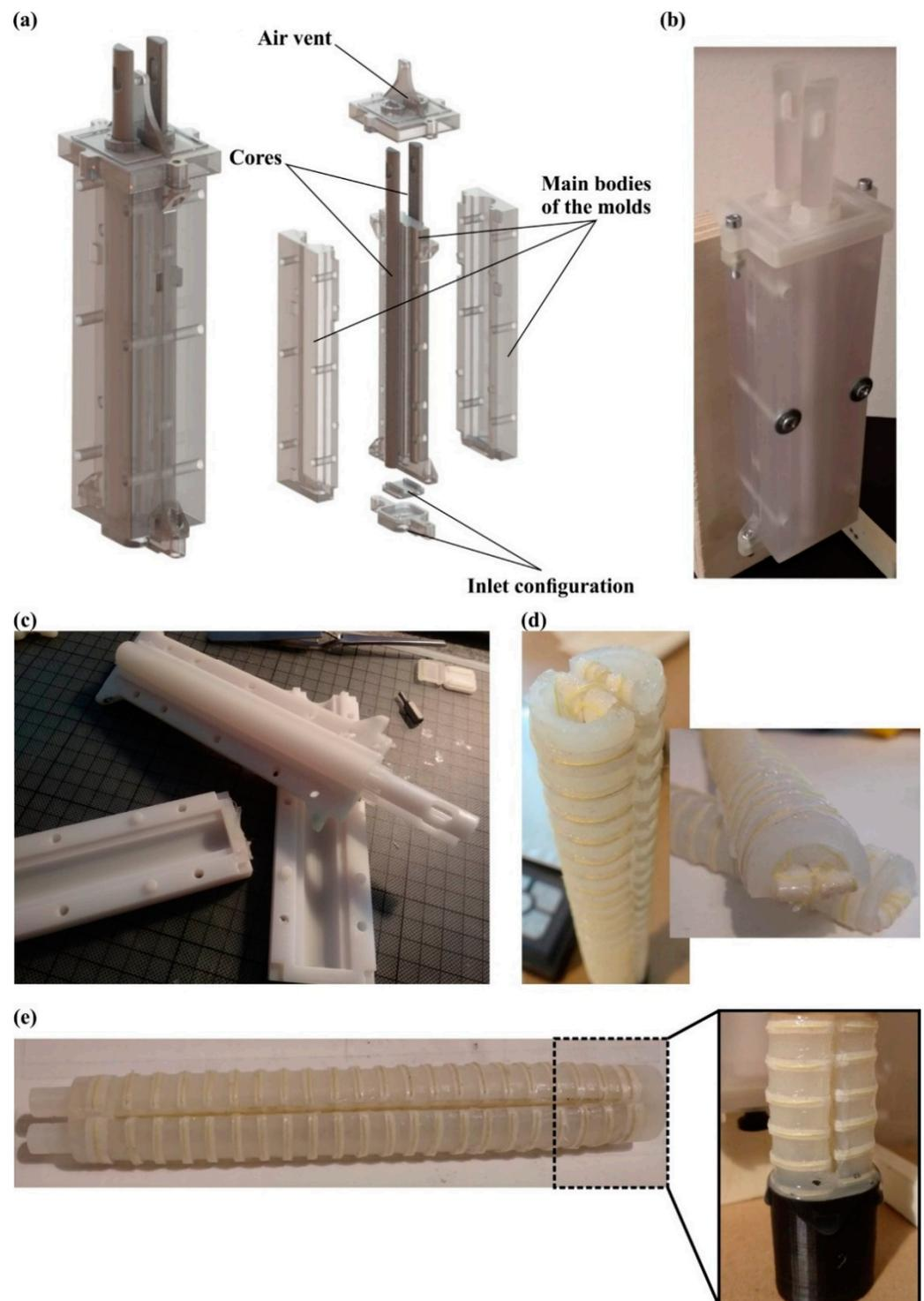
**Figure 3.** (a) A 3D model and exploded view of the silicone molds; (b) Image of the 3D printed mold; (c) Releasing process of the pneumatic chamber from the molds; (d) Indicative Kevlar reinforcement of the pneumatic chambers; (e) Bonding and final design of the soft actuator.
