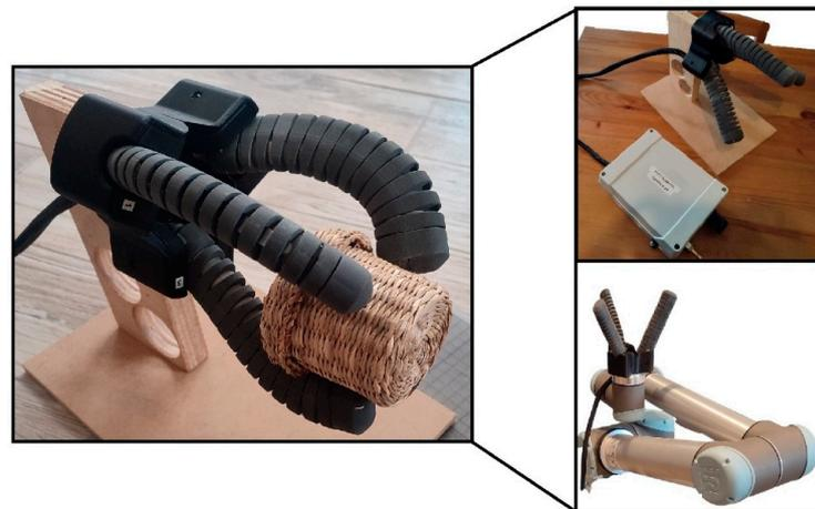
**Figure 9.** Indicative applications for the developed actuator: (a) Exoskeleton for medical applications to assist patients with mobility difficulties; (b) Soft gripper for the handling of delicate objects.
