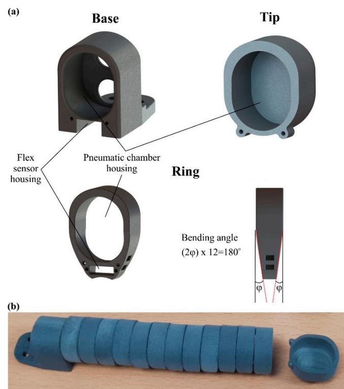
**Figure 4.** (a) 3D models of the base, ring, and tip; (b) 3D printed external covers made of PA12.
