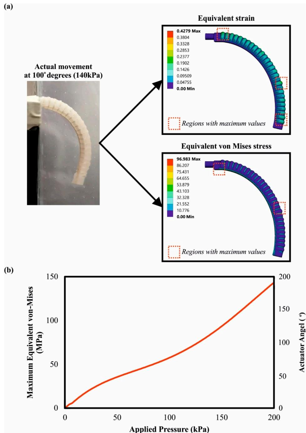
**Figure 8.** (a) Indicative images of the actuator’s motion derived from the physical testing and the FEA; (b) Graphical relations between the applied pressure, the bending angle, and the developed von Mises stress on the actuator.
