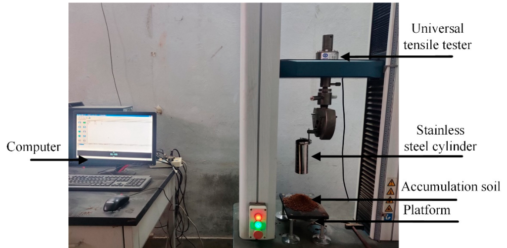
Figure 5. Soil repose angle test device.
