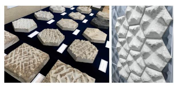
**Figure 16.** Left: Photograph of the cumulative textures of the various investigations, and right: The assembly of a potential application using P1 prototype.
