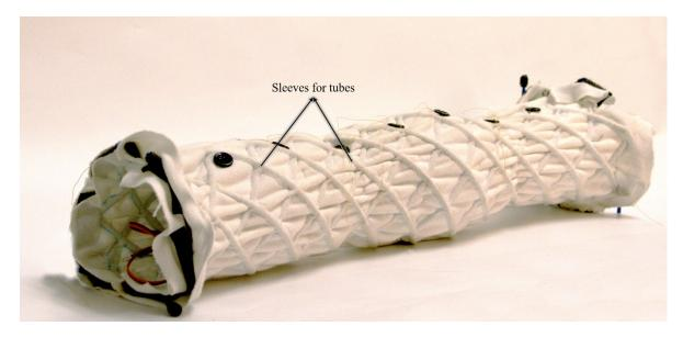
**Figure 6.** The MiniFabricWorm consists of no rigid components in the structure. The sleeves through which tubes pass are visible. The length of MiniFabricWorm in its rest state is 55 cm.
