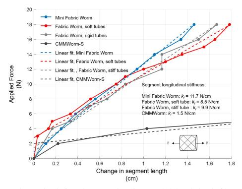
**Figure 8.** Change in length of a single segment when a force is applied along the length of the segment. The slope of the linear fit (dashed lines) of the curves is used to estimate the longitudinal stiffness of the segment.  $k_l$ : Longitudinal stiffness; *F*: Force applied in the horizontal direction.
