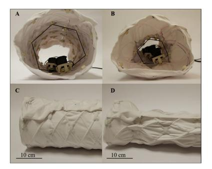
**Figure 5.** FabricWorm in different actuation phases. (**A**) Front view of FabricWorm fully expanded. The actuation cable is highlighted (black hexagon drawn over the cable for visibility). (**B**) As the actuation cable (smaller black hexagon) is spooled-in, the robot contracts in diameter. (**C**) Side view of fully expanded FabricWorm. (**D**) Side view of fully contracted FabricWorm.
