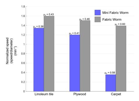
**Figure 11.** Robot speed normalized by diameter for FabricWorm with stiff tubes (gray) and MiniFabricWorm (blue). A video was taken from the sagittal view and Tracker software was used to measure the progress made over time for both robots on substrates with different coefficients of friction (indicated on top of each bar). The MiniFabricWorm robot was run three times over multiple wave cycles on linoleum tile and plywood, and twice on carpet.  $\mu_s$ : Coefficient of static friction.
