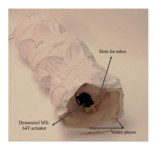
**Figure 4.** FabricWorm during a peristaltic wave. The various components of the structure are labelled. The sleeves through which the tubes pass can be seen on the inside of the fabric. The total length of FabricWorm in its rest state is 67 cm.
