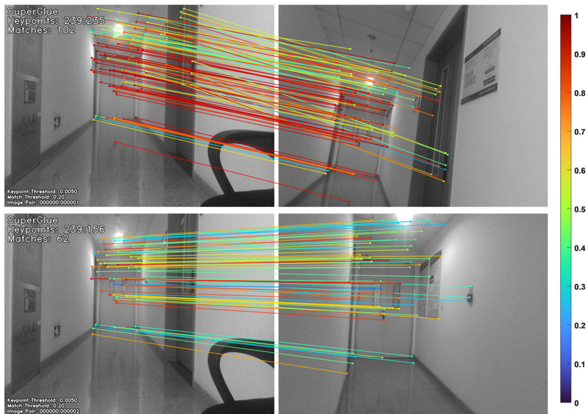
Figure 2. Feature extraction and matching results. The lines in the figure represent feature point pairs, and the colors represent confidence levels.
