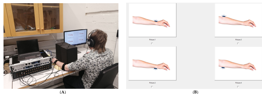
Figure 1. (A) The experimental setup, showing the wearable vibrotactile bands with actuators positioned on the forearm. (B) The response screen; observers clicked on the image depicting the site they thought had been stimulated (see Section 2).
