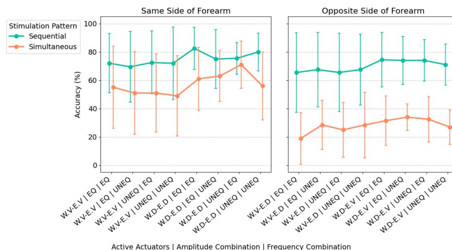
Figure 2. Recognition accuracy across simultaneous and sequential stimulation modes for the different actuator locations (W.V, Wrist. Volar; W.D, Wrist. Dorsal; E.V, Elbow. Volar; E.D, Elbow. Dorsal), amplitude, and frequency combinations (EQ, Equal; UNEQ, Unequal) on the same and opposite side of the forearm. Points indicate the mean recognition accuracy. Error bars represent \pm 1 standard deviation (SD).
