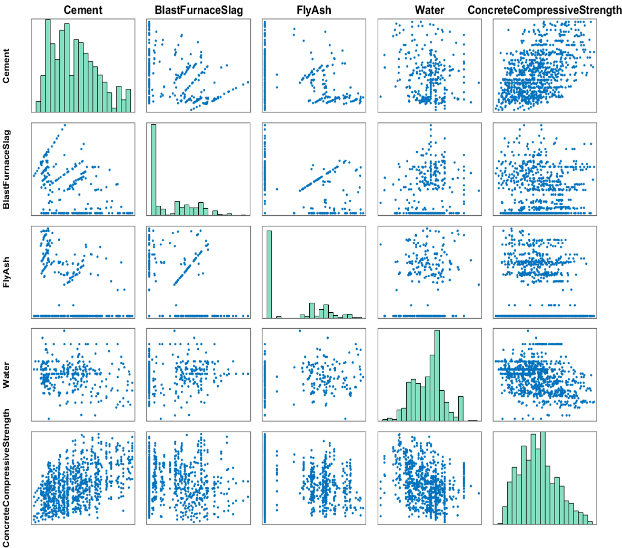
Figure 5. The relationship graph between concrete strength and the initial 4 input features: cement, water, fly ash, and blast furnace slag.
