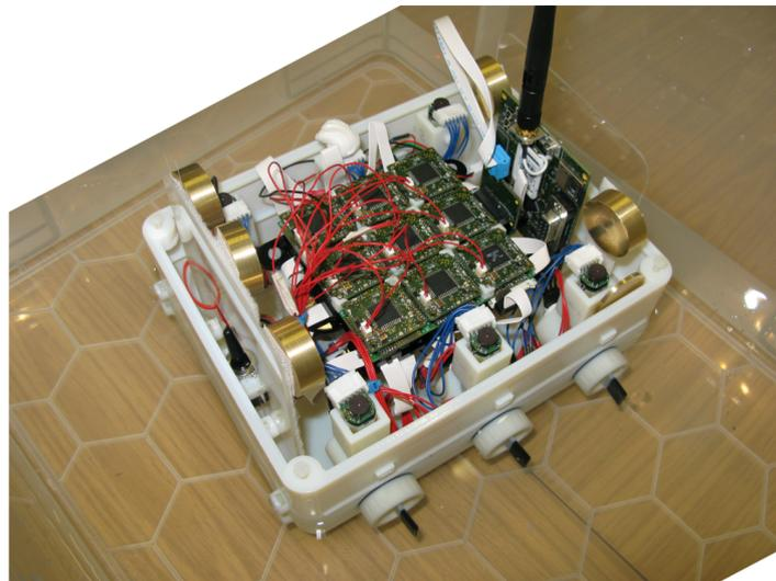
**Figure 1.** Physical platform. The physical cellular automata (CA) architecture is connected to six independent paddlers provided with Encoder and index hall effect sensor. It is powered by a three-cell lithium battery.
