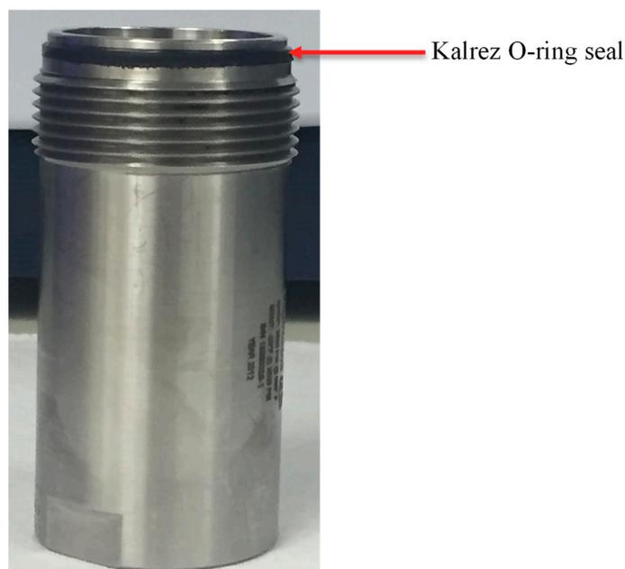
**Figure 2.** A photograph of the autoclave cell showing the position of the O-ring elastomer.
