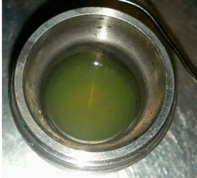
**Figure 4.** Glycol appearance inside the autoclave cell after the O-ring failure.
