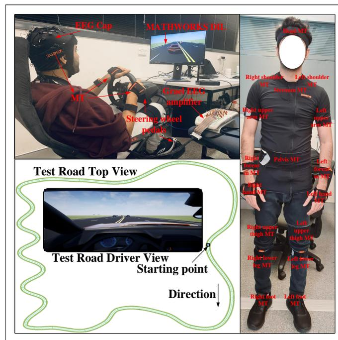
**Figure 2.** MATHWORKS DIL platform and deployment of 17 MTs on various body parts.
