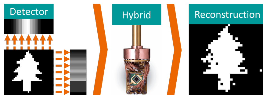
Figure 1. Graphical Abstract: Simulation and reconstruction of a two-view binary tomographic problem using hybrid quantum annealing.
