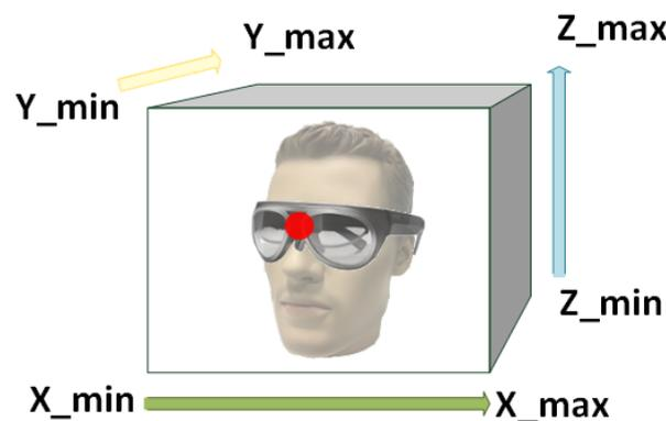
**Figure 5.** Prediction relative to object box. The predicted translation (red) is relative to a predefined object box. The borders of this box have been determined as the minimum and maximum translation values per axis based on the ground truth annotations.
