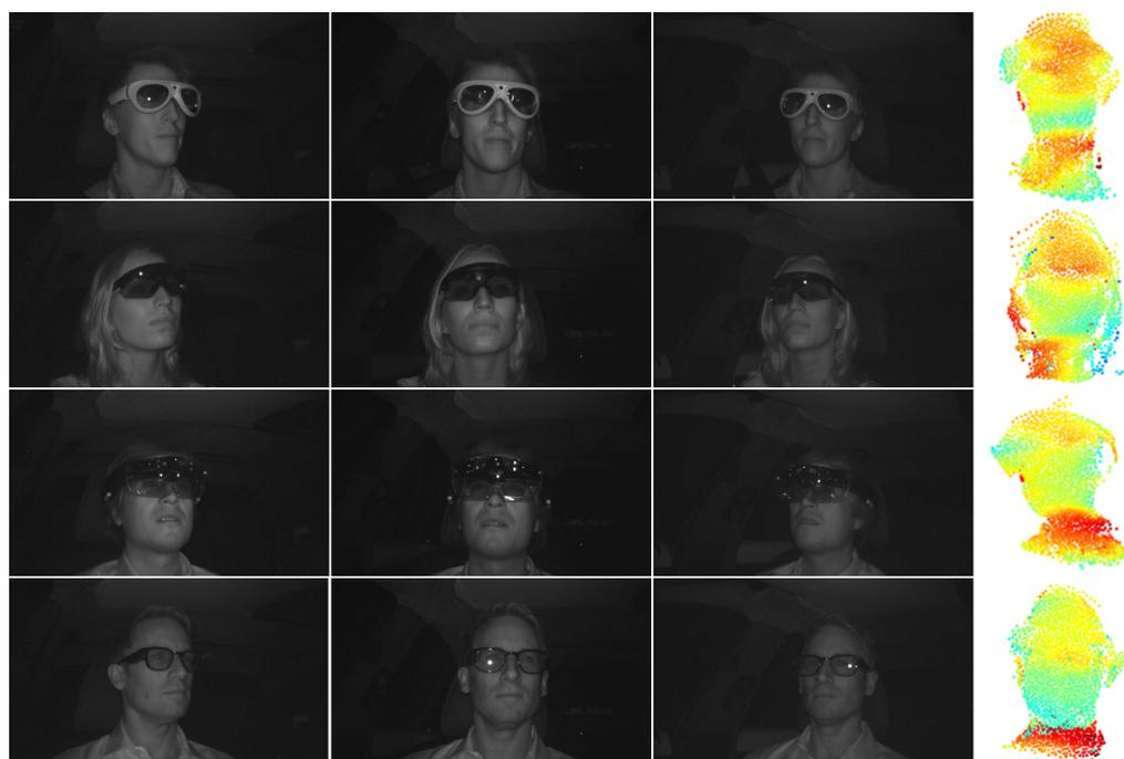
**Figure 6.** Four example triples with the estimated point cloud, predicted by the central image only. Each row visualizes an example triple for a different person, wearing different glasses and the corresponding point cloud. The lighter the blue color of 3D point, the more the relative distance of a particular 3D point.
