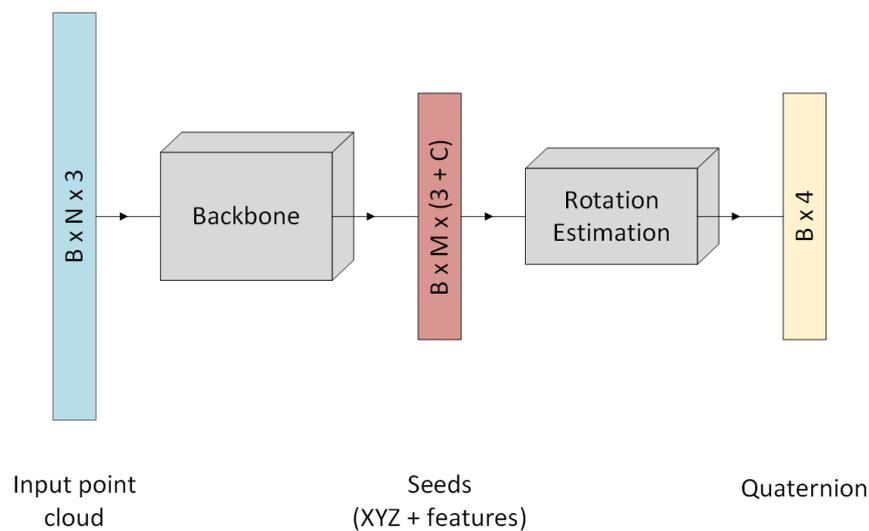
**Figure 7.** Overview of P2R-Net architecture. N is the number of points, B refers to the batch size of the network, M is the number of seed points and C is the number of additional features found by the network.
