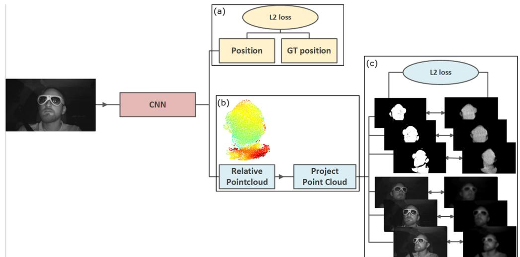
**Figure 2.** An overview of our overall architecture. (a) We estimate the translation based on the ground truth. (b) The point cloud estimation is performed with self-supervision based on (c) pre-generated masks of the target objects and the intensities of the original images.
