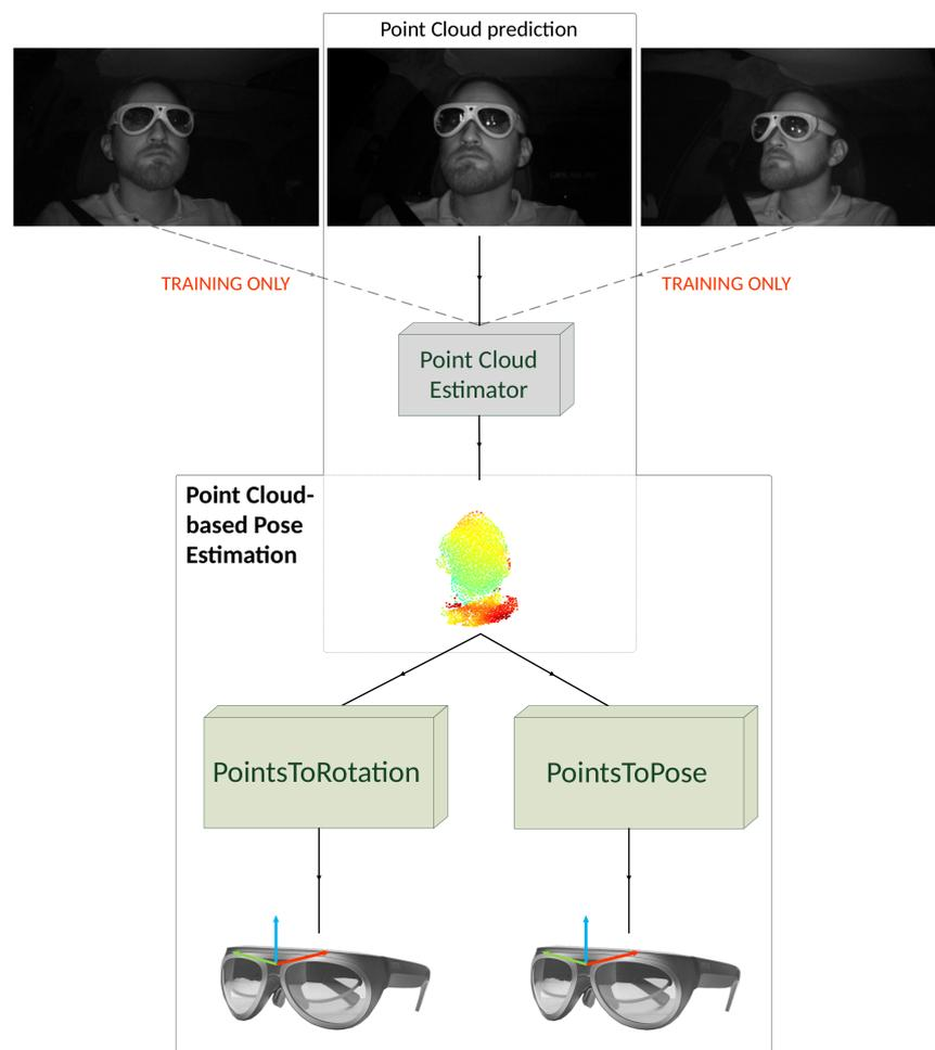
**Figure 1.** Our full object pose estimation pipeline. We train our point cloud estimator on three images and need one image during testing only to predict a point cloud. We use the point cloud for both our pose estimation methods.
