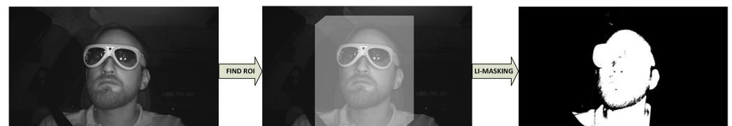
**Figure 3.** Mask generation pipeline. From left to right: determine region of interest based on projection of rendered cuboid and Li-Thresholding.
