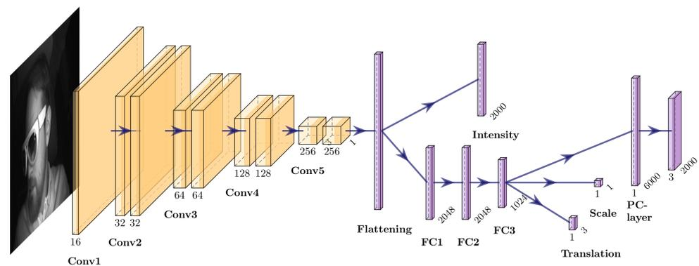
**Figure 4.** An overview of the CNN architecture. We use convolutional layers to extract features from the input image. The number of filters is doubled per convolutional block. The kernel size changes between one and three, starting with three in the first layer of the first convolutional block. While color information is directly regressed from the flattened feature vector, a decoder processes the feature vector before scale, translation and point cloud are predicted.
