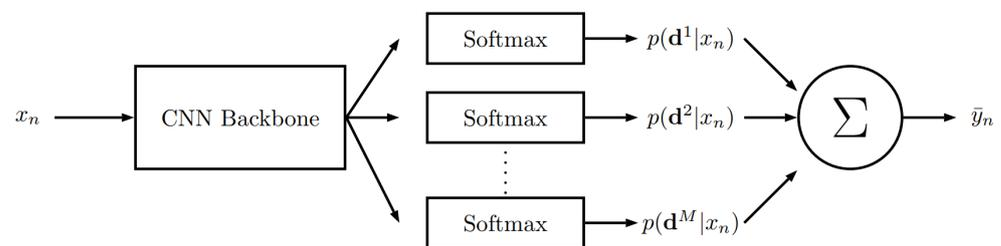
**Figure 9.** Overview of the RvC-based pose estimation method [6].  $p(d^M|x_n)$  depicts the softmax layer outputs per class  $D^m$  for an input  $x_n$ . The outputs are being combined using an ensemble average to obtain a final pose estimation.
