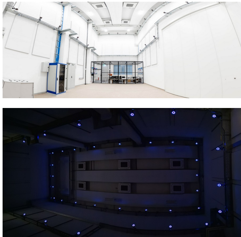
Figure 3. Pictures of our drone hall with the motion capture system used for our pipeline. With a set of 37 cameras we are able to track the hall's complete volume. The second image is taken upward to capture as many cameras as possible and to showcase the available tracking volume. (Top) picture reprinted with permission from Daniel Waschnig. Copyright 2019 Daniel Waschnig. (Bottom) picture reprinted with permission from Fred Arneitz. Copyright 2019 Fred Arneitz.
