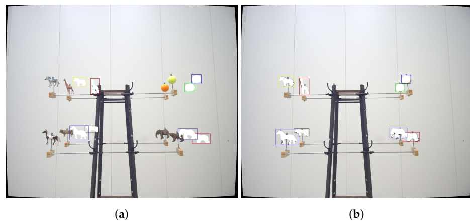
Figure 9. Comparison of the annotation quality for an image annotated using different extrinsic calibrations. (a) (Manual extrinsic calibration) shows the annotation result using a manually determined extrinsic calibration between camera image plane and camera tracking rigid body. Given the marker configuration from Figure 4a, we manually measured the transformation from the pivot marker to the assumed position of the image sensor. In (b) (Optimized extrinsic calibration), the results are presented for the extrinsic calibration determined by solving the optimization problem. In general, determining the correct extrinsic calibration between rigid body and image plane greatly improves the annotation quality. Best viewed as PDF and in color.
