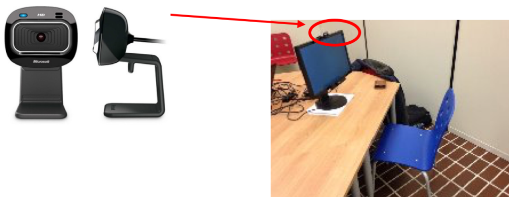
Figure 3. Eye-tracking device and subject's position in front of the screen for eye-tracking acquisitions.
