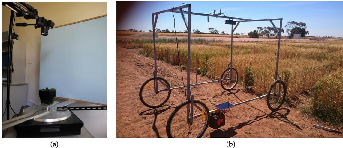
**Figure 1.** This figure shows the two imaging platforms we have build in house for imaging plants. (a) is the platform for imaging plants indoor and (b) is the platform for imaging outdoor plants growing in field condition.
