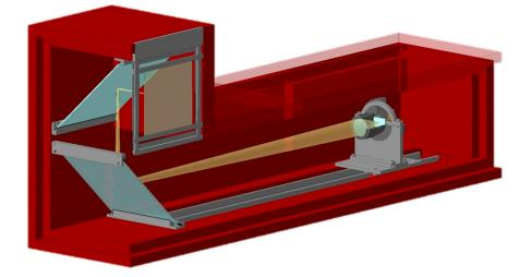
**Figure 2.** Scheme of the detector system used on the neutron radiography and tomography facility on the IBR-2 reactor. Firstly, the neutron radiation is converted into light photons by a scintillator plate. The scintillator thickness is 100  $\mu$ m. The light from the scintillator is reflected by the mirrors, and then directed to the optical system of the high resolution and high sensitive CCD-based video camera.
