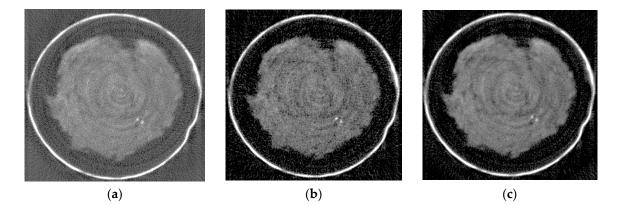
**Figure 3.** The examples of the tomography slices of the golden vial reconstructed by the conventional FBP algorithm (**a**), by the SIRT reconstruction with 150 iterations (**b**), by the SART algorithm with 150 iterations (**c**).
