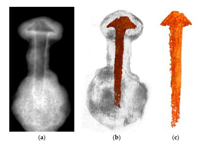
**Figure 4.** (a) The neutron radiography image of the fragment of the bireme remains; the background is black; (b) the virtual 3D model of the fragment of the bireme remains, the copper remains are labeled in a dark yellow color, the corrosion component is grey; the corrosion components are made more transparent for clarity; (c) the separated 3D volume of the metal inclusion in the bireme fragment.
