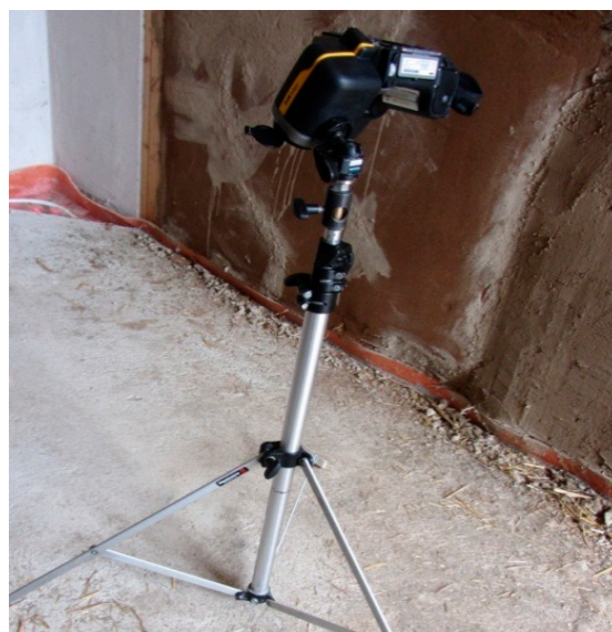
Figure 4. The infrared camera facing the radiant floor.
