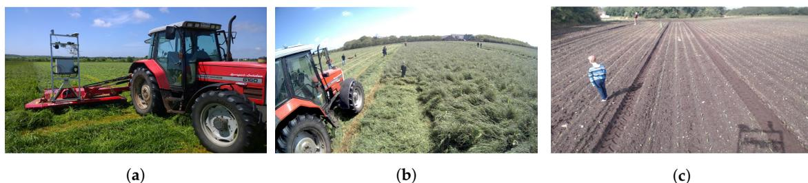
Figure 2. Images from experiments and recordings. (a) The sensor kit mounted on a mower; (b) An example image from the recordings in grass; (c) An example image from the recordings in row crops.
