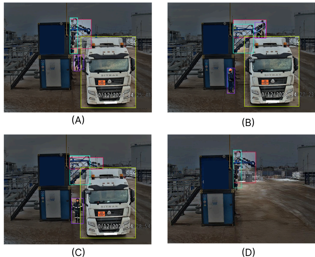
Figure 6. Events of the oil product filling process: (A) the event of the tanker truck arrival stage; (B) the event of the tanker truck preparation stage; (C) the event of installation of the overhead filling device in the tankers; (D) the events of the tanker truck departure stage.
