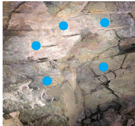
Figure 18. Schematic diagram of rebound hammer testing in hard rock zones.
