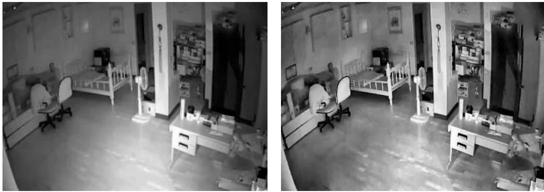
Figure 2. Images before and after adaptive histogram equalization.
