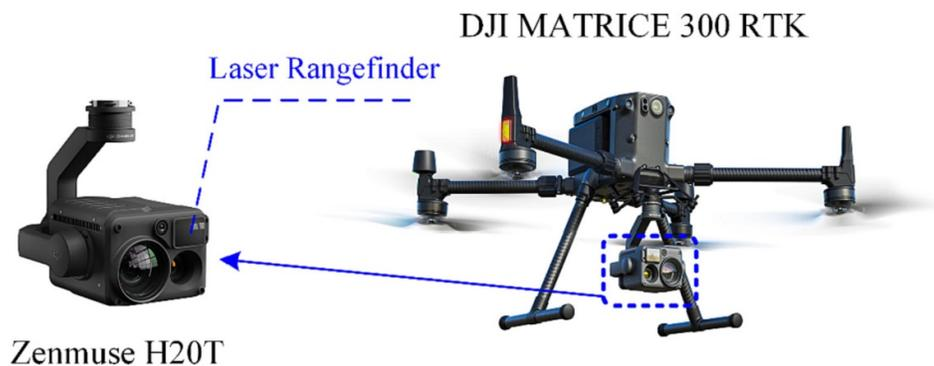
**Figure 2.** Components of UAV. Reprinted with permission from ref. [50]. Copyright 2023 Elsevier.
