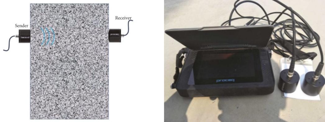
**Figure 5.** Ultrasonic concept on concrete (left) with the Pundit PL-200 sonicator (right). Adapted from [82].
