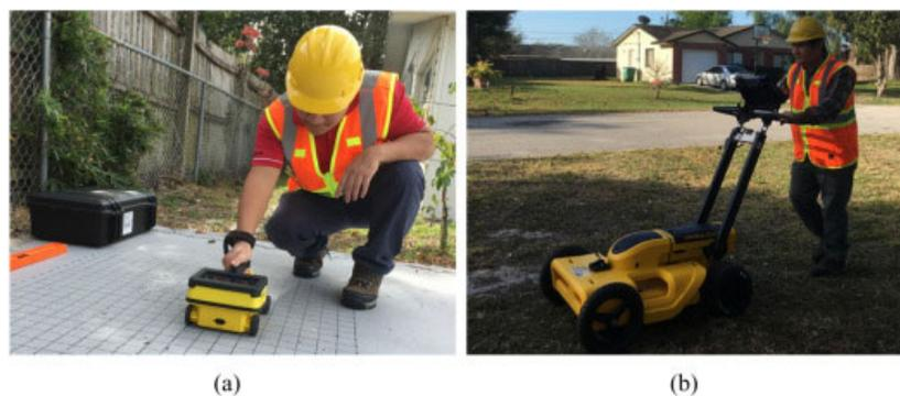
**Figure 6.** Using GPR for (a) concrete scanning and (b) utility locating. Reprinted with permission from ref. [83] Copyright 2021 Elsevier.
