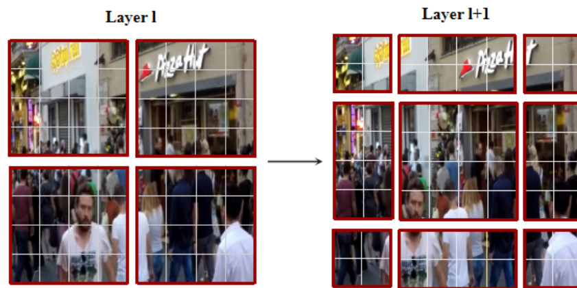
Figure 4. Regular local window partition and shifted window partition.
