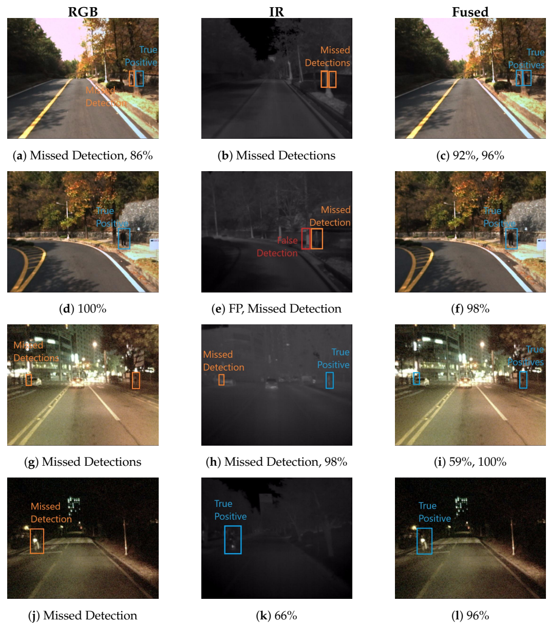
Figure A1. Additional qualitative comparison of results: Missed and false positive detections are represented by orange and red bounding boxes, respectively, while blue bounding boxes indicate accurate detections in accordance with the ground truth. Improved detection accuracy can be observed in the multimodal domain compared to missed detections in the visual domain.
