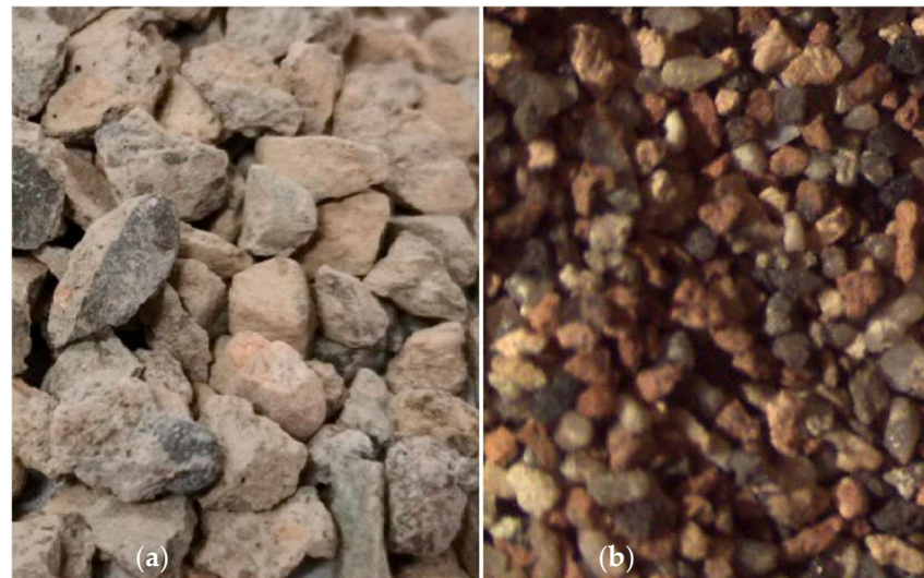
Figure 2. Recycled coarse aggregates studied in 3DPC; (a) recycled concrete [29] and (b) recycled brick [28].
