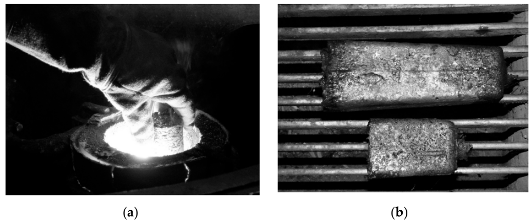
Figure 13. (a) Charging of compact into melt. (b) Ingots composed of basic steel and added compacts [186].
