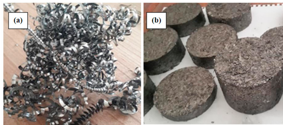
Figure 12. (a) The Ti6Al4V chip, and (b) the briquettes pressed from their chip [136].
