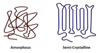
Figure 3. Arrangement of molecules in amorphous polymers and semi-crystalline polymers [24].
