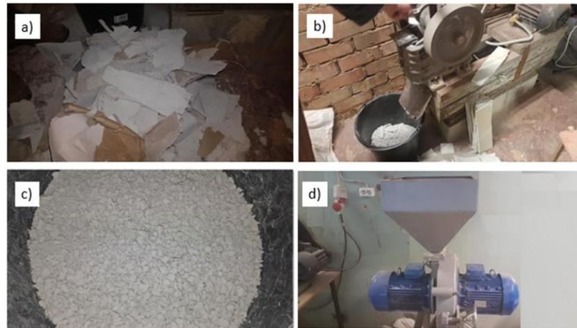
**Figure 1.** The treatment process of CDW to obtain secondary gypsum powder for binder production: (a) collection of gypsum wallboard CDW; (b) crushing of wallboards with laboratory jaw crusher; (c) gypsum CDW aggregate (<11.2 mm) prepared for milling; (d) gypsum CDW milling in disintegrator (collision milling).
