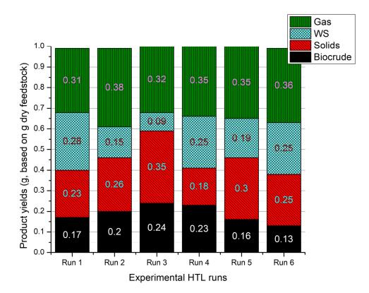
**Figure 3.** Overview of HTL product yields, including biocrude, solids, water solubles and gases, indiscriminately scaled to a closed mass balance.
