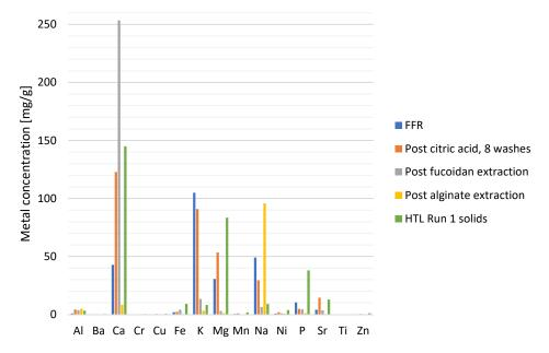
**Figure 5.** Comparative metal concentrations in raw macroalgae, citric acid leaching, fucoidan, and alginate extraction residues, and the solids produced in HTL run 1, as determined by ICP ash analysis.
