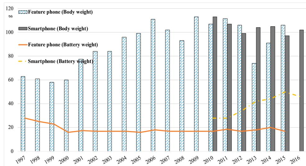
**Figure 7.** Average body and battery weight for each type of WMPs.
