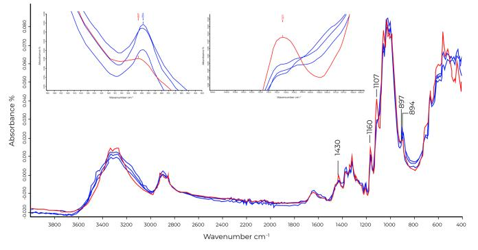
**Figure 3.** Full FTIR spectra of merceried pre-consumer samples in blue and reference 100% cotton sample in red; enlarged FTIR spectra of mercerised pre-consumer samples in blue, and reference 100% cotton sample in red with a change from 897 cm<sup>-1</sup> to 894 cm<sup>-1</sup> (top left); enlarged FTIR spectra of mercerised pre-consumer samples in blue, and reference 100% cotton sample in red: disappearance of the cotton peak in the mercerised samples at 1107 cm<sup>-1</sup> (top right).
