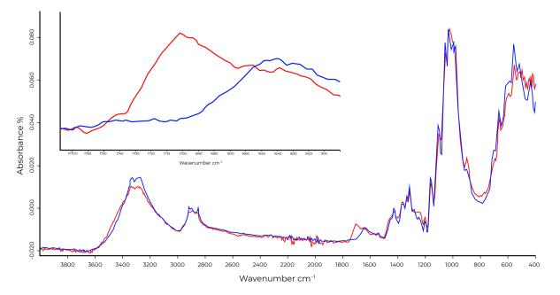
**Figure 2.** Full FTIR spectra of a pre-consumer cotton sample (blue) compared to a post-consumer cotton sample (red) with changes caused by dialdehyde formation on the cellulose by oxidation; enlarged FTIR spectra of a pre-consumer cotton sample (blue) compared to a post-consumer cotton sample (red) with changes caused by dialdehyde formation on the cellulose by oxidation: a change in the area of  $1700-1730 \text{ cm}^{-1}$ .
