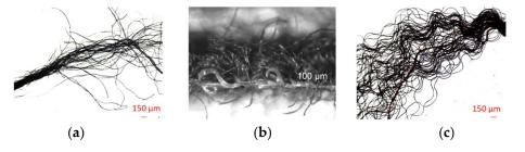
**Figure 1.** Microscope images of elastane-containing materials (**a**) cotton yarn where elastane was in the core of the yarn; (**b**) knitted cotton textile where elastane is fed backside of the fabric; and (**c**) polyester filament yarn including elastane.
