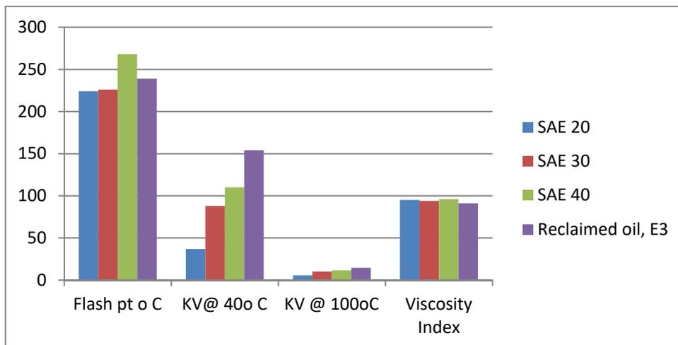
Figure 5. Comparison between SAE20, SAE 30, SAE 40 and reclaimed oil (E3).
