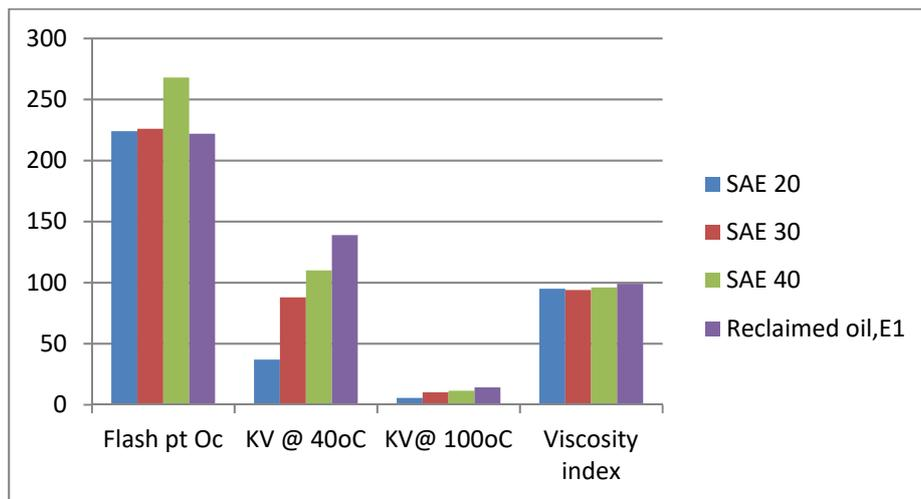
Figure 3. Comparison between SAE 20, SAE 30, SAE 40 and reclaimed oil (E1).
