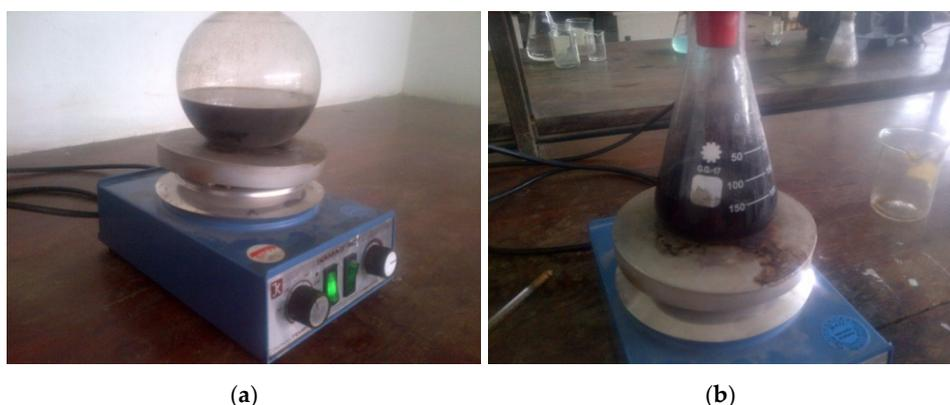
**Figure 1.** (a) Solvent extraction and (b) Adsorption process with activated charcoal.
