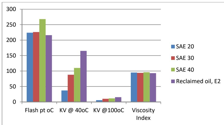
Figure 4. Comparison between SAE20, SAE 30, SAE 40 and reclaimed oil (E2).
