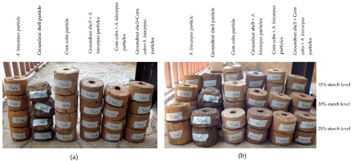
Figure 2. (a) Briquettes produced based on particle types; (b) Briquettes produced based on particle types and starch levels.
