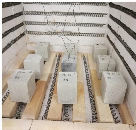
Figure 4. View of cubic samples before temperature loading, thermocouple fixing.
