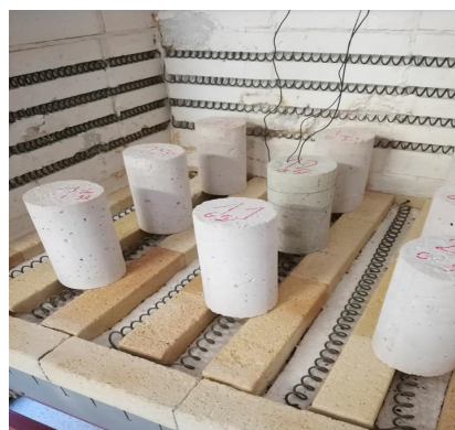
Figure 3. View of cylindrical samples before temperature loading, thermocouple fixing.
