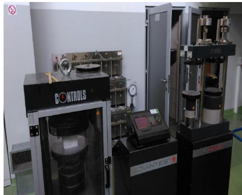
Figure 2. View of the Controls Advantest 9 hydraulic press adapted to test compressive strength.
