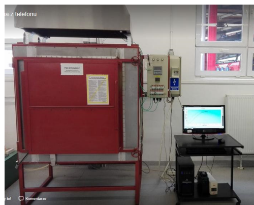
Figure 1. View of the PK 1100/5 chamber furnace with instrumentation.
