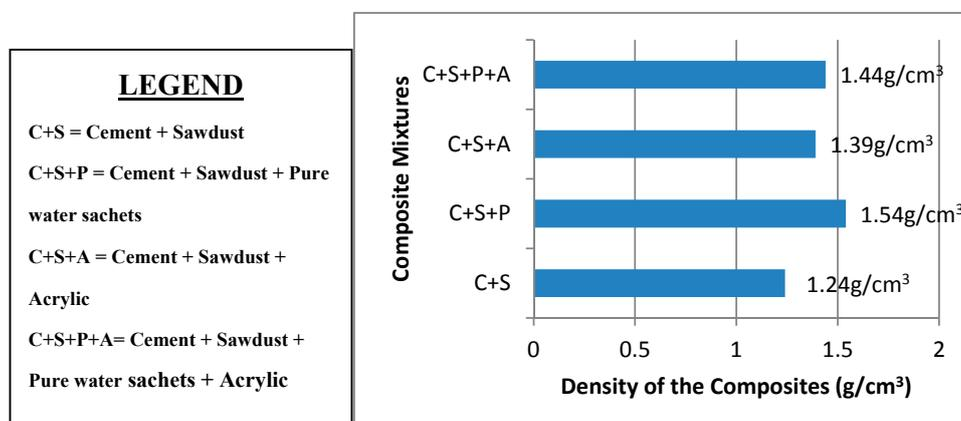
Figure 5. Density of the composites.
