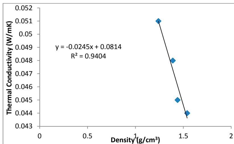
Figure 11. Correlation between density and thermal conductivity of the composites.
