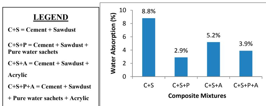
**Figure 6.** Water absorption of the composites.
