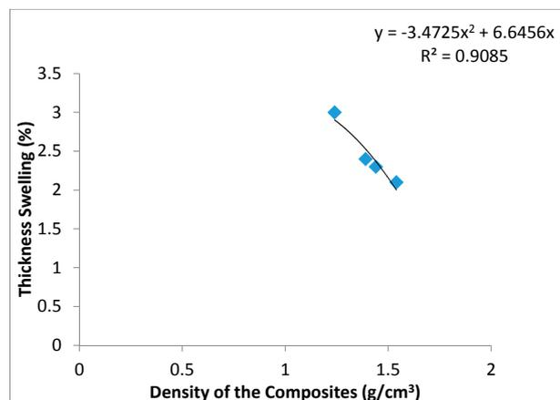
**Figure 9.** Correlation between density and thickness swelling.
