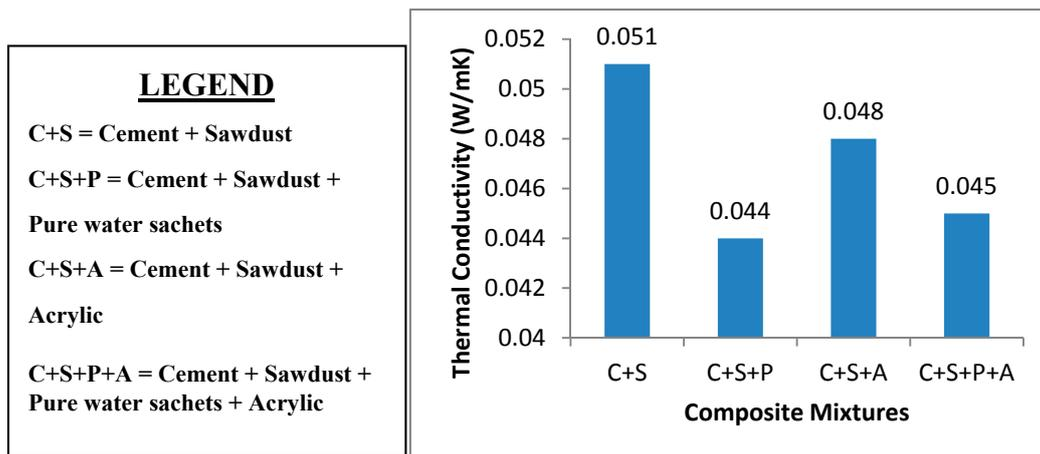
Figure 10. Thermal conductivities of the composites.
