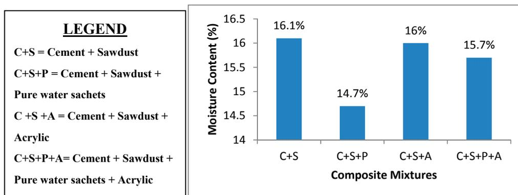
Figure 4. Moisture content of the composites.
