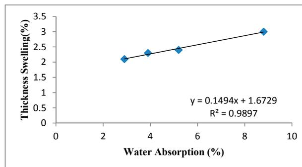
**Figure 8.** Correlation between water absorption and thickness swelling.
