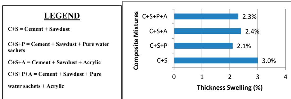
**Figure 7.** Thickness swelling of the composites.
