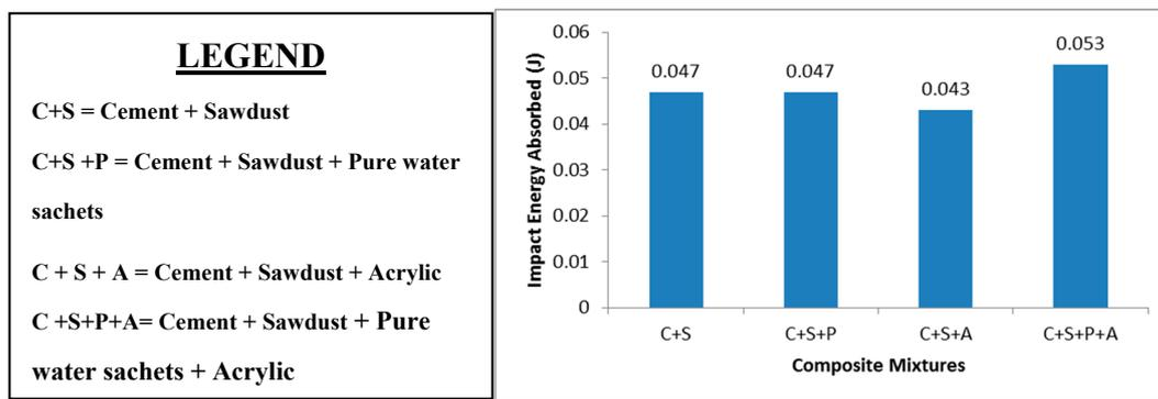
Figure 12. Impact energy of the composites.
