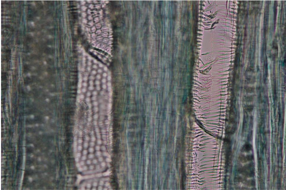
**Figure 25.** Tangential view of face veneer showing alternate intervessel pitting, spiral thickenings, and cross section of sample perforation plates (400 $\times$ ) that are characteristic of sugar maple (*Acer saccharum*).
