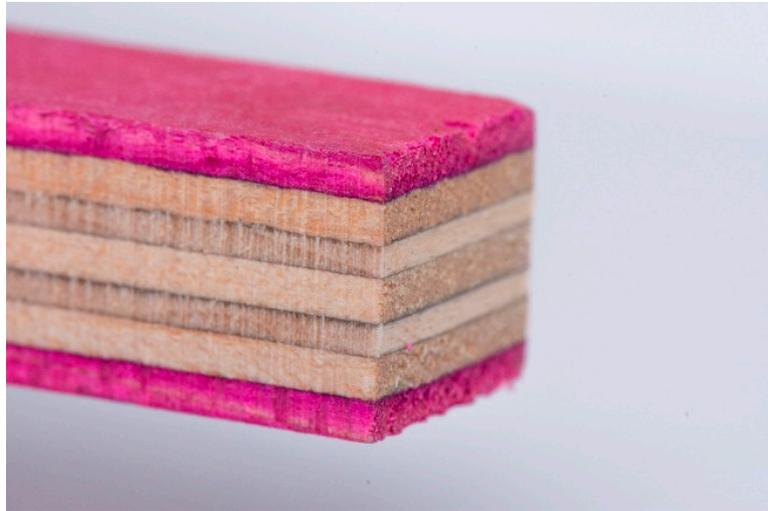
**Figure 7.** Face Wise Strip Orientation.
