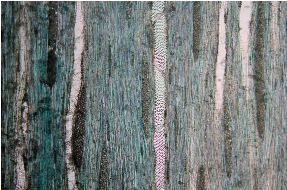
**Figure 26.** Tangential view of face veneer showing alternate intervessel pitting, spiral thickenings, and cross section of sample perforation plates (100 $\times$ ) that are characteristic of sugar maple (*Acer saccharum*).
