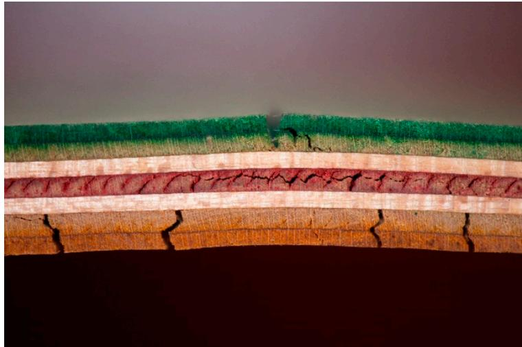
**Figure 18.** Cross Section View Showing Splitting in Sample 3.
