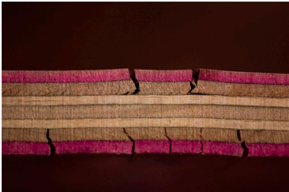
**Figure 17.** Cross Section View Showing Splitting in Sample 2.
