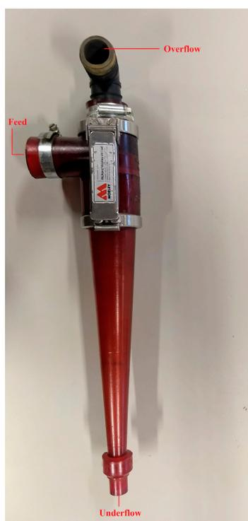
**Figure 1.** A typical hydrocyclone (Image taken by Malik Degri).
